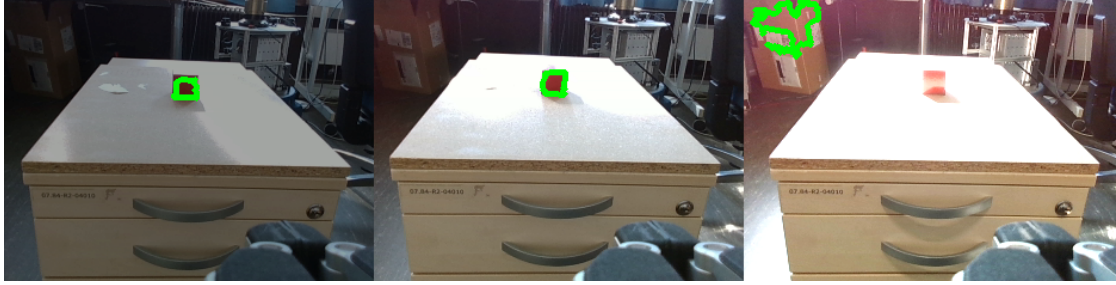
Figure 5.6: Cube tracking in three more complex lighting scenes. A dark scene with reduced brightness on the left, soft oblique light in the middle and very strong direct sunlight to the cube on the right.
