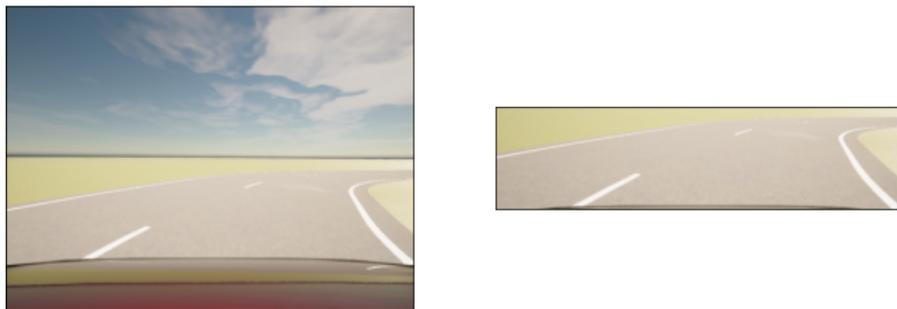
Figure 3.4: Example image with a resolution of 800x600x3 (width x height x channels) from Data Set (left) - cropped and scaled image only containing relevant parts of the image used for training with a resolution of 200x66x3 (right).
