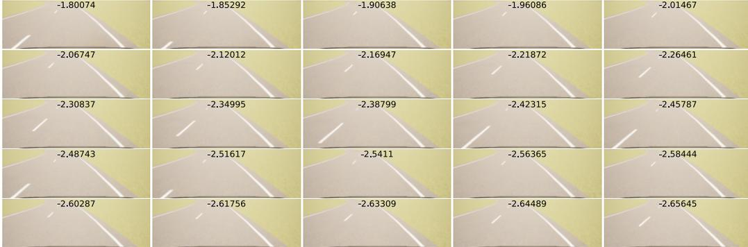
Figure 3.2: 25 frames long excerpt of generated data ordered line-by-line showing the vehicle's alignment to the target trajectory.
