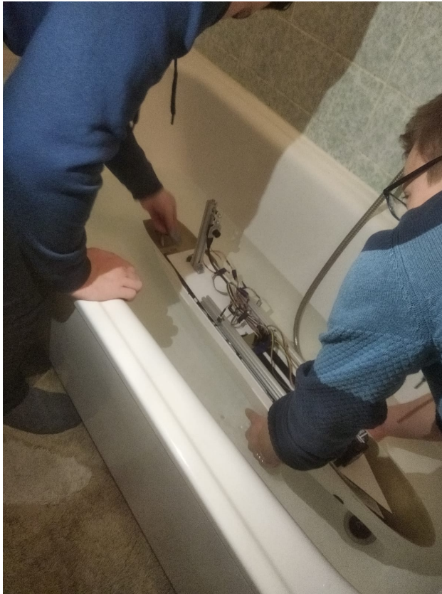
Figure 9.1: The first watering of the ship. Fortunately only a small amount of trimming was needed to keep it stable.
