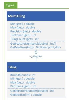
**Abb. 4.4: MultiTiling in RLLibrary .NET**
